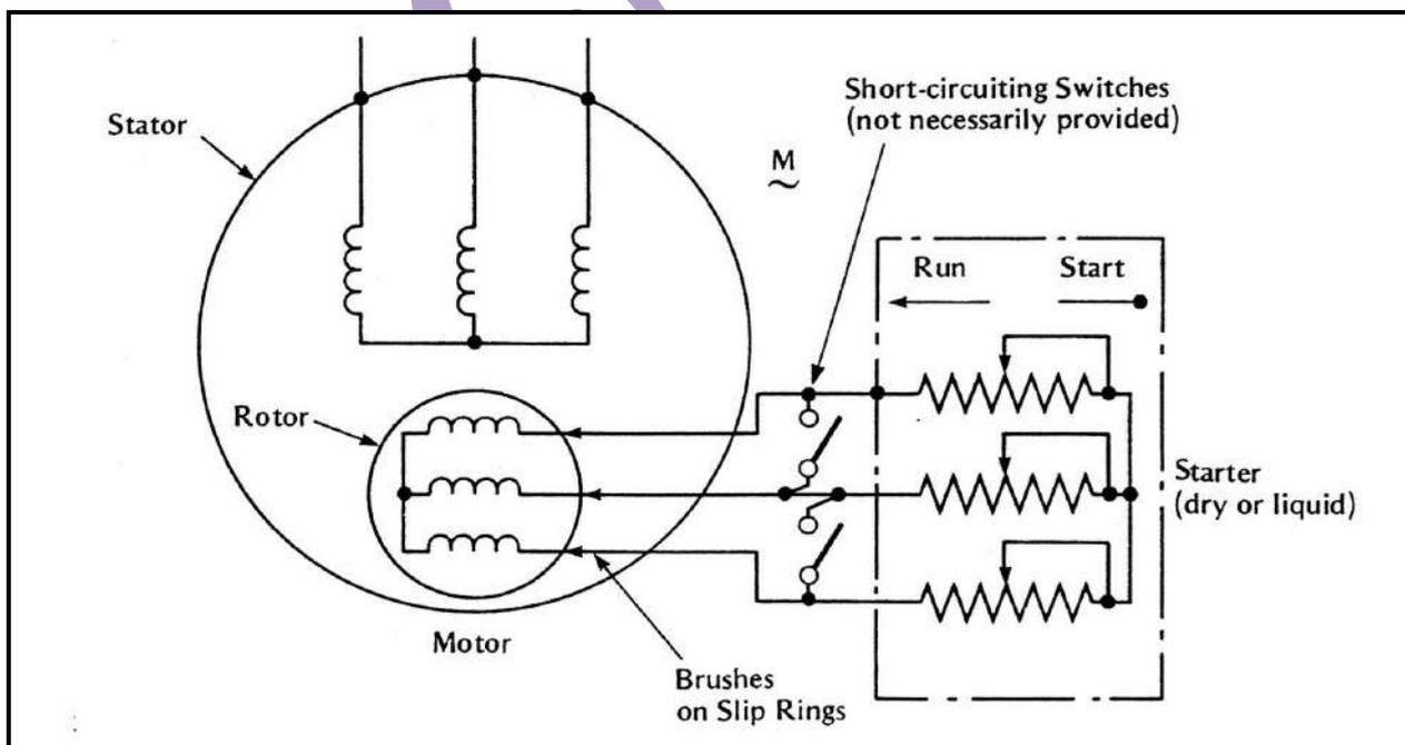
**FIGURE 9.1: SLIPRING MOTOR STARTER**
